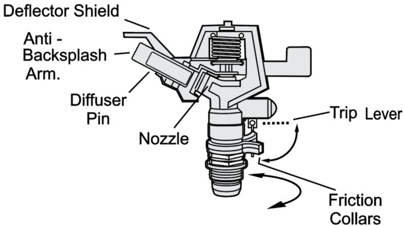
Figure 2: An impact rotor sprinkler.
